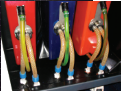
Heating lines on wax ink tanks
